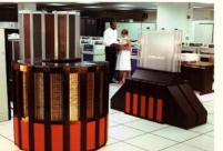
Cray 2 supercomputer (1985) 1.9GFlops
