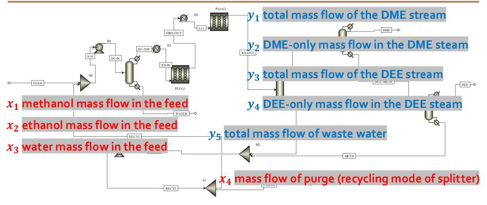
a chemical plant that uses methanol, ethanol, and water to manufacture dimethyl ether (DME) and diethyl ether (DEE)
